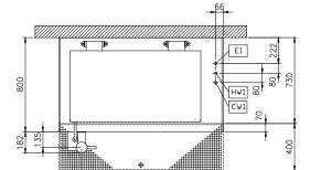
Cold Water inlet 1 (cleaning) Electrical inlet (power) Hot water inlet
